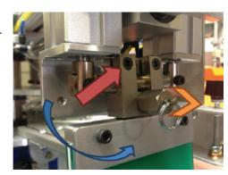
4. In this picture, the blue arrow is pointing to the chopper cylinders. There is one chopper cylinder on each side of each print head. Both correspond with the squeegee pressure. Tighten to increase pressure on your squeegee.
